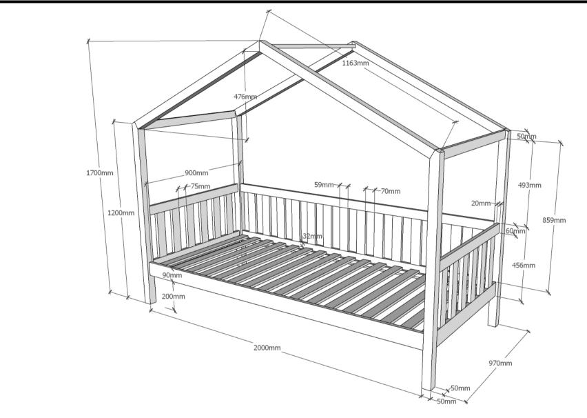
L:2100mm H:1700mm D:970mm innersize 900x2000mm
